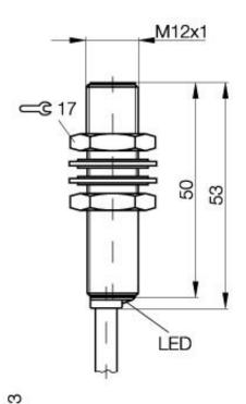
**Inductive Sensors** BES M12MI-NSC20B-BV03 M12x1 x 53 normally-open Sn=2mm shielded
